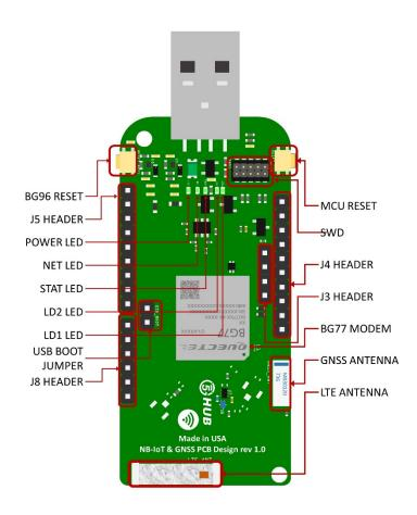
Figure 4. USB Dongle Top Side – Key Components
