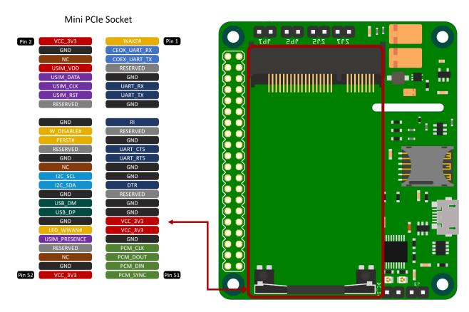
Figure 3. miniPCle Pin Assignment
