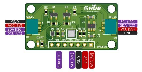
If used with the NB-IOT board as below, connect the **SCL**, **SDA**, **GND**, **VCC** lines in the two boards together.
