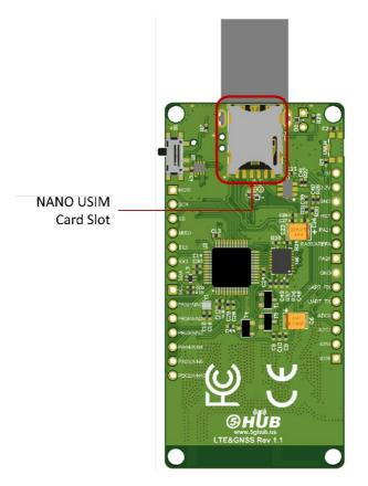
Figure 5. USB Modem Bottom Side – Key Components
