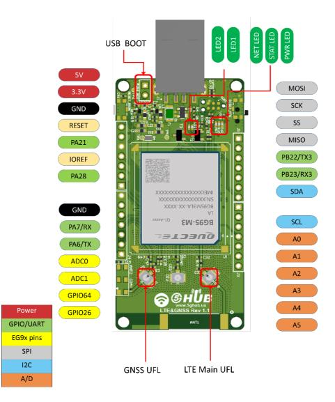
Figure 4. USB Modem Top Side – Key Components
