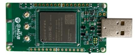
Figure 1. USB Modem Overview Diagram – Top View
