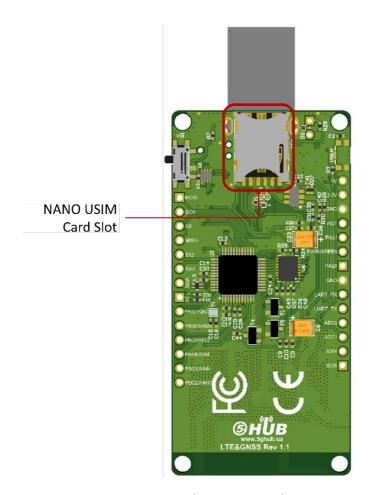
Figure 5. USB Modem Bottom Side
