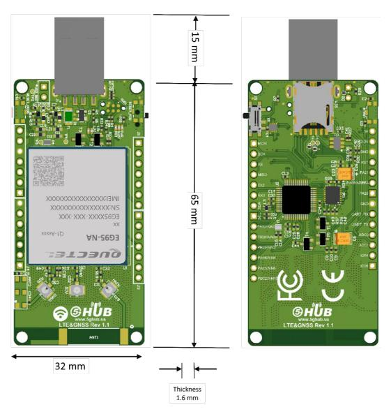
Figure 3. Physical Characteristics.
