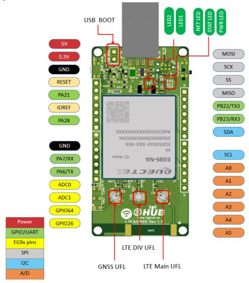
Figure 4. USB Modem Top Side (EG9x)
