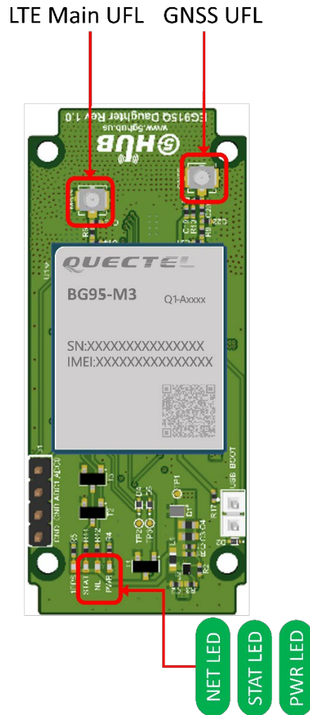
Figure 4. Daughterboard Top Side – Key Components
